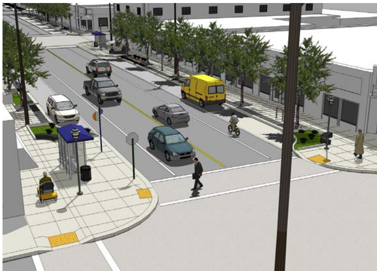
AT CERTAIN “SPECIAL” INTERSECTIONS, PEDESTRIAN CROSSWALKS WILL BE TREATED WITH THE SAME CONCRETE USED WITHIN THE CLEAR ZONE OF THE SIDEWALK. WHERE THIS OCCURS WITHIN STREETS WITH TEXTURED PAVERS, THE EDGE OF THE CROSSWALK SHALL BE BORDERED WITH CONTRASTING PAVERS TO THOSE USED WITHIN THE TRAVEL LANE
